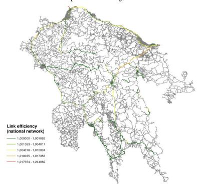
Figure 10: Link efficiency in the national road network of Peloponnesus
